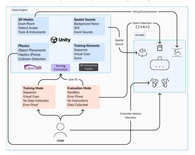
Figure 1. Conceptual design and system architecture of NursingXR.
