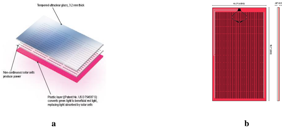
Fig 1: Wave length selective PVs, b- The lower luminescent layer, (LUMO PANEL – soli-culture, 2020)
