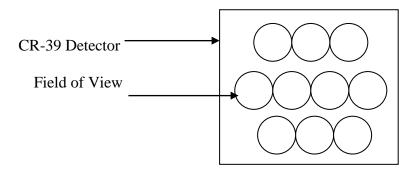
Figure 3. Schematic Representation of Field View on the Surface of the Detector
