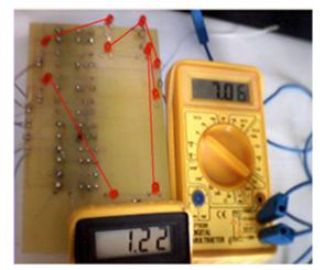
Fig. 1 A virtually wired real circuit in the AR remote lab leads to AR based visualization.
