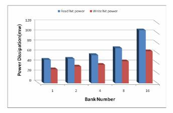
Figure 7: Read and write hitt power results for various cache's bank number.
