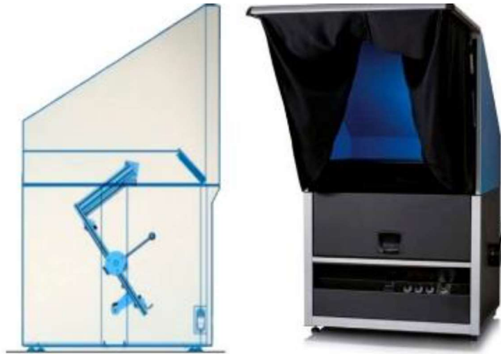
Figure 1: The Byko-spectra effect light booth (BYK-Gardner). The left image shows the inner structure and the rotation platform of the light booth.
