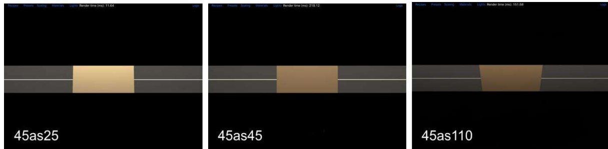
Figure 3: Screenshots of the rendering on the iPad of color-only simulation of a flat metallic coating panel inside the virtual light booth at three different geometries.
