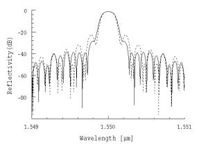
Figure 4: Reflectivity spectra for segmented Gaussian apodized normal FBGs with maximum error of 0.014 (solid line) and 0.08 (dashed line).
