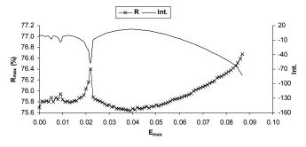
Figure 2:The maximum reflectivity and the integration of the error as a function of maximum error for approximated Gaussian apodized FBGs
