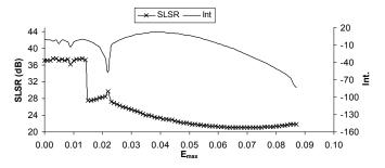
Figure 3:The SLSR and integration of error for the approximated Gaussian apodized FBGs as a function of error.
