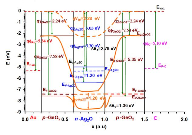
Figure 1: the energy band diagram for the GeO<sub>2</sub>/Ag<sub>2</sub>O/GeO<sub>2</sub> heterojunctions
