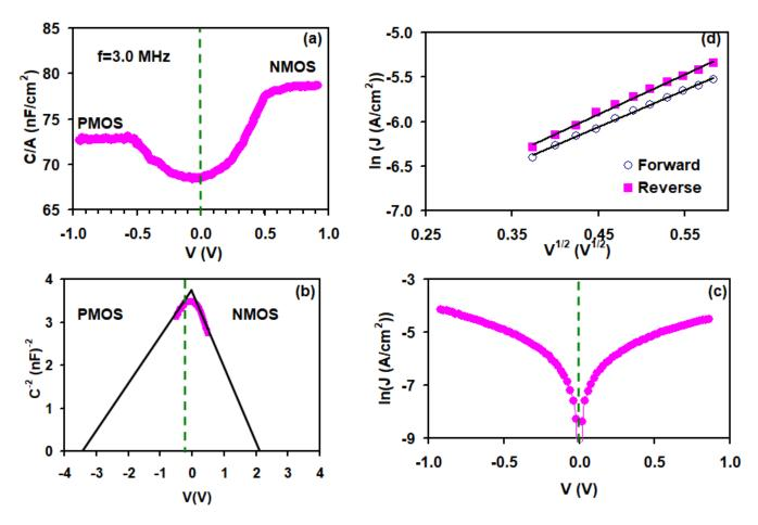
Figure 7: (a) the capacitance-voltage characteristics, (b) the  $C^{-2} - V$  variations, (c) the current-voltage characteristics and (d) the  $\ln(I) - \sqrt{V}$  variations for Al/GeO<sub>2</sub>/Ag<sub>2</sub>O/GeO<sub>2</sub>/C devices.
