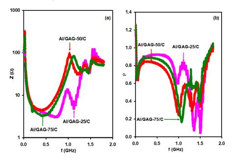
Figure 5: (a) the impedance and (b) the reflection coefficient spectra for  $Al/GeO_2/Ag_2O/GeO_2/C$  devices.
