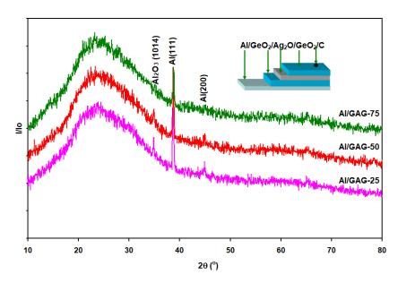
Figure 2: The X-ray diffraction patterns for the stacked layers of  $GeO_2$  comprising  $Ag_2O$  nanosheets. The inset shows the geometrical design of the studied devices.
