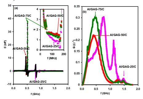
Figure 4: (a) the capacitance and (b) the conductance spectra for Al/GeO<sub>2</sub>/Ag<sub>2</sub>O/GeO<sub>2</sub>/C devices. The inset of (a) show the variation of the exponent s of the equation,  $G \propto F^s$ . The black colored circles in (a) represent the fitting of Eqn. (1).
