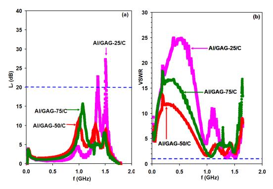
Figure 6: (a) the return loss spectra and (b) the voltage standing wave ratios for the  $Al/GeO_2/Ag_2O/GeO_2/C\ devices.$
