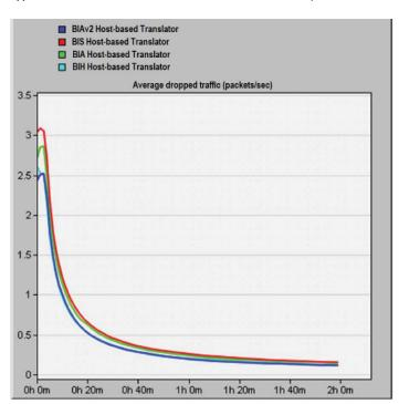
Figure 15. Average dropped traffic for BIS, BIA, BIH, and BIAv2 host-based translators (from Site A to Site B)
