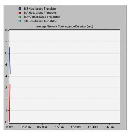
Figure 17. The duration of network convergence when using host-based translators
