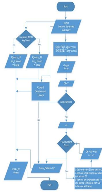
Fig. 4 Query Pattern Extraction Algorithm
