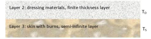
**Figure 2.** Three-layer model for dressed burn wound comprising of: a semi-infinite layer of air, finite thickness layer of dressing materials, and a semi-infinite layer of burn-damaged skin.
