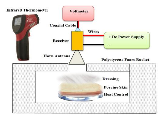
**Figure 3.** Experimental setup for the emissivity measurements of the porcine skin samples. A digital voltmeter is used to measure the output voltage level of the samples and a thermocouple and an infrared thermometer are used to measure the thermodynamic temperature of the samples.
