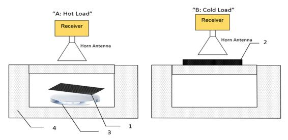
**Figure 4.** Radiometric emission centered at 90 GHz is collected by a moveable horn antenna at positions: A to measure a hot calibration source (1) (carbon loaded foam absorber; type: Eccosorb AN-73) stabilized at a temperature ~54 °C using a digital hotplate (3) placed in a polystyrene foam bucket (4), B to measure the cold calibration source (2) (carbon loaded foam absorber; type: Eccosorb AN-73) in thermodynamic equilibrium with air temperature ~20 °C.
