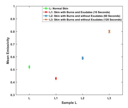
**Figure 10.** Mean emissivity values and standard deviation bars for porcine skin sample before and after different applications of localized heat treatments. L represents the normal skin; L1 represents skin with burns and exudates after 10 s of heat treatment, L2 represents skin with burns and without exudates after 60 s of extra heat treatment, L3 represents skin with burns and without exudates after 120 s of extra heat treatment.
