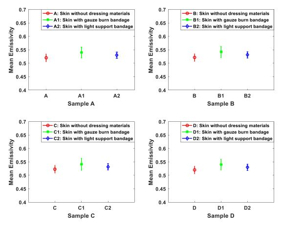
**Figure 7.** Mean emissivity values and standard deviation bars for porcine skin without and with dressing materials. The samples A, B, C, and D represent skin without dressing materials, A1, B1, C1, and D1 represent skin with six-layer gauze burn bandage, and A2, B2, C2, and D2 represent skin with a light support bandage.
