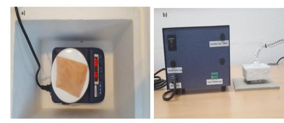
**Figure 5.** A digital hotplate used for heating and stabilizing the surface temperature of the porcine skin samples (a) and a heat control device with  $(50 \times 50 \text{ mm})$  metal plate used for performing burns on the porcine skin samples (b).
