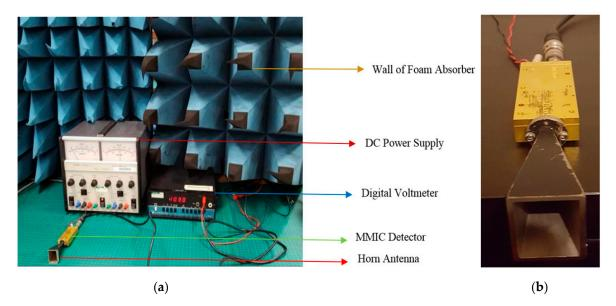
**Figure 3.** (a) Experimental setup showing the horn antenna and the MMIC detector. The detector was connected to a digital voltmeter and a DC power supply. A wall of anechoic chamber is surrounding the majority of the system. (b) The radiometer.
