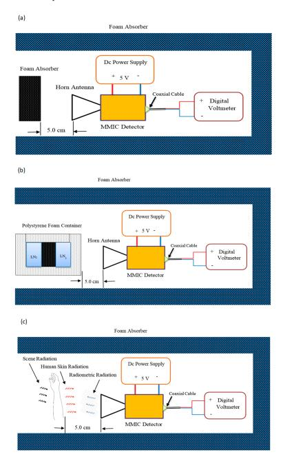
**Figure 4.** Schematics of the experimental setup inside the walls (blue-grey) of the anechoic chamber, showing the hot (a) and the cold (b) calibration procedures and the measurement of the skin (c).
